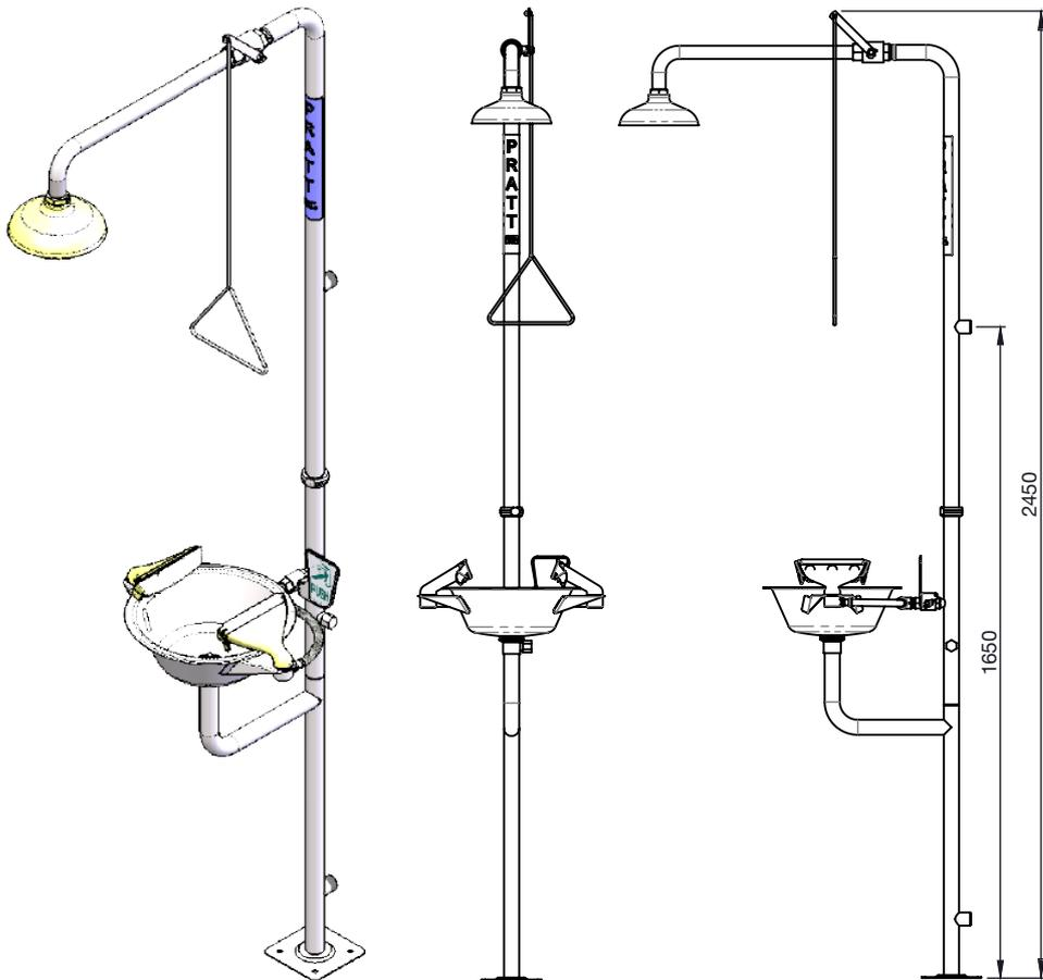
**Inlet and Outlet Connections: 25mm BSPM**
